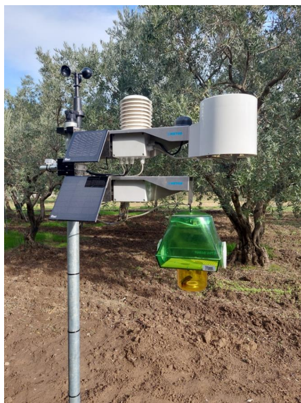
Figure 35. Digital traps and weather station installed in the LL
