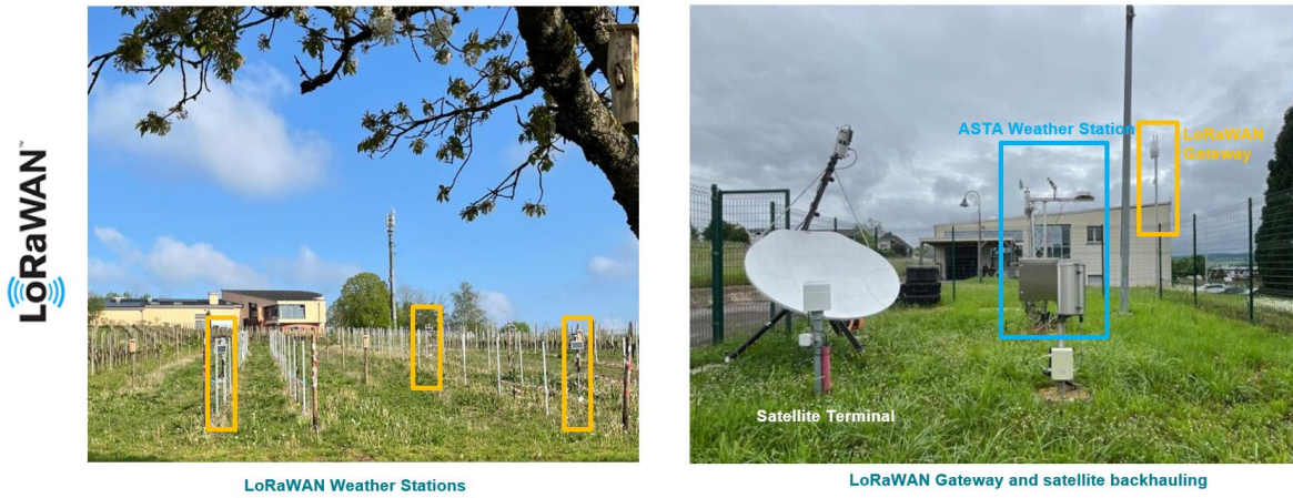
Figure 7: LoRaWAN based deployment in the LL at IVV Remich
