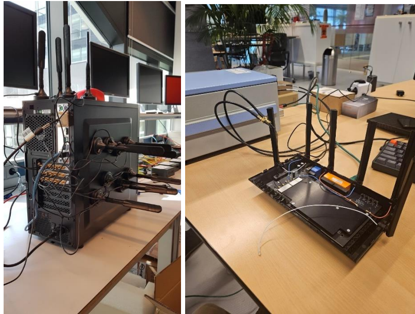
Figure 47. Amarisoft's 5G node (left) and TP-Link's WiFi node (right)
