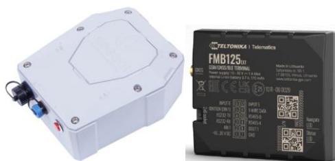
Figure 49 LoRaWAN gateway and GPS tracker
