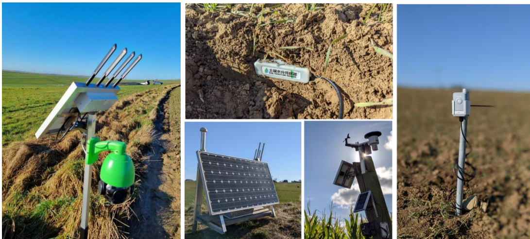
Figure 2: 5G camera and LoRa Devices (Soil-Moisture Sensors and Weather station)
