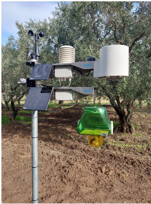
Figure 18. A soil-plant-atmosphere sensor station, including soil sensors and weather data acquisition sensors.
