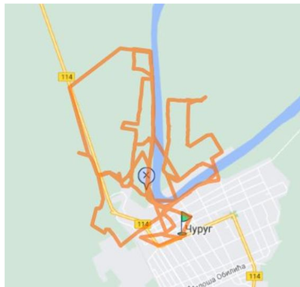
Figure 21. LoRaWAN gateway location and covered route.
